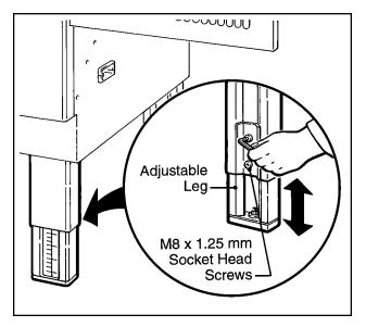
Figure 2-4 – Conveyor Bed Height Adjustment
